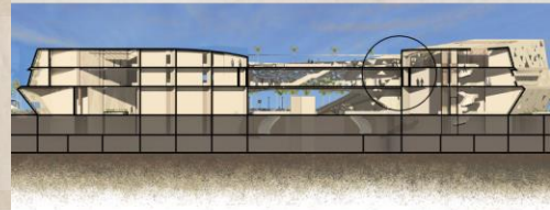
A metal decking system was used, supported by two columns on each side to reinforce the bridge structure.
