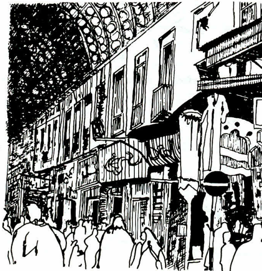
Fig. 8. The use of arcades, colonnades, small enclosed top-covered courtyards, streets will alleviate the harshness of the lack of humidity in a hot-dry climate [8, p.67].
