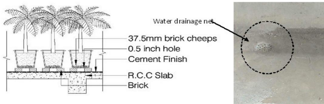
**Figure 3:** Section of pot plants arrangement (Left) and net on water drainage pipe (Right)
