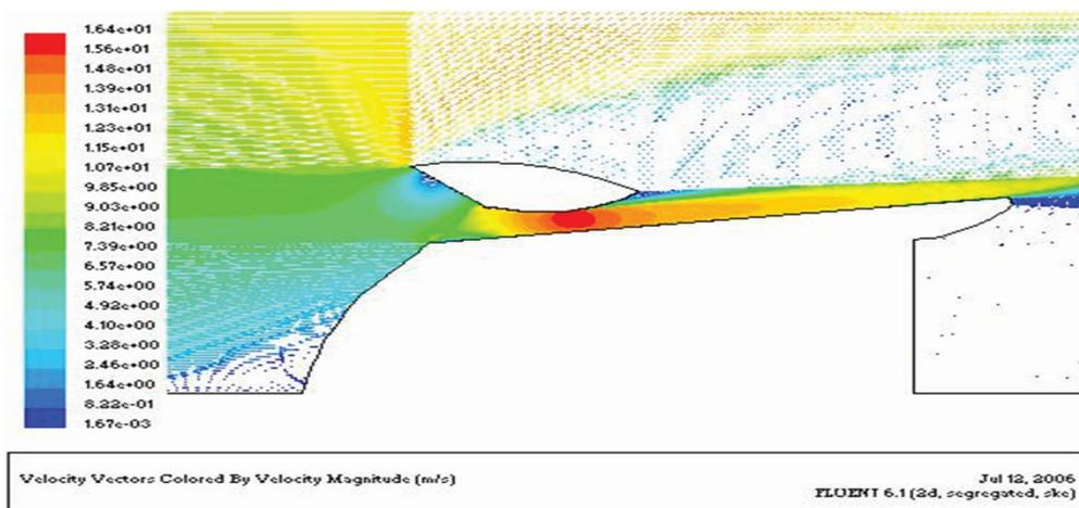
Figure 22: Velocity vectors for wing front angle of attack 40°, in a large grid case.
