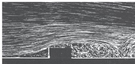
Figure2 2: Visualisation of the turbulent separation at the leading roof edge of a flat roof.
