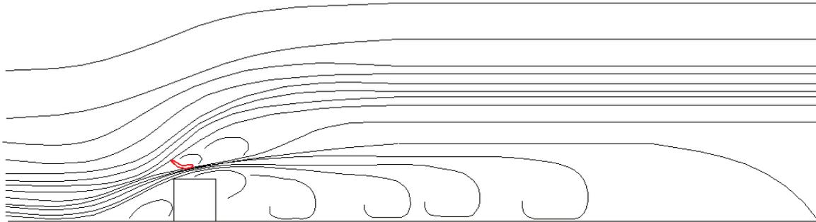
Figure 6: Flow separation after installing a wing shape on top of a building.
