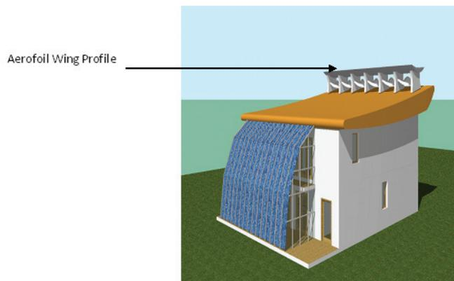
Figure 9: Typical wind turbine integrated in a prototype-detached house, Wing profile on high end of the roof.
