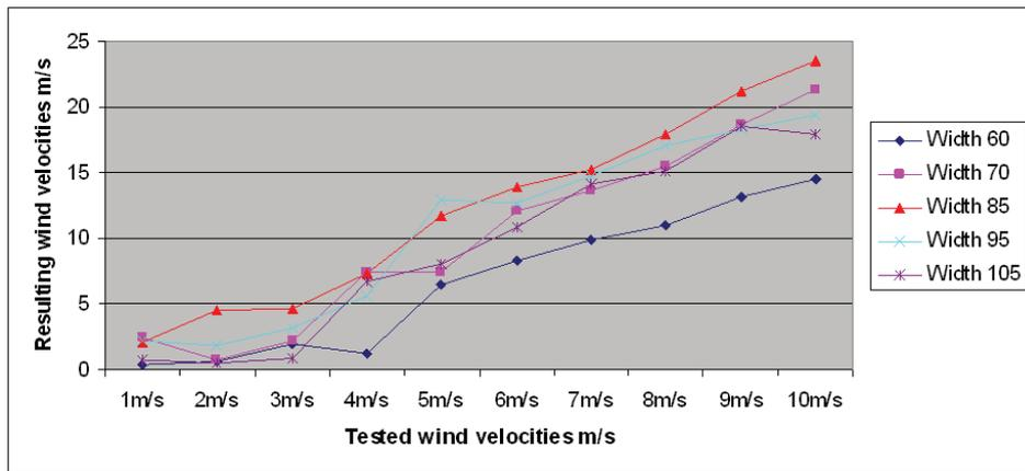
Figure 15: Summary of different proximities of the wing to the roof and its effect of velocity. generated.
