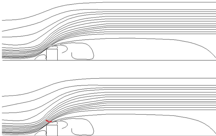
Figure 3: Flow schematic sketch, with areas of re-circulation in front, top and back of the building (left to right).
