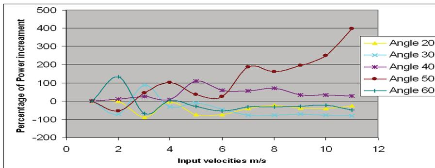
Figure 26: Percentage of power increment as the angle of wing increases.
