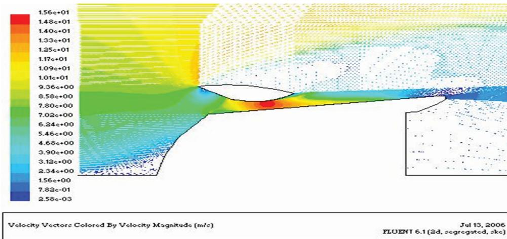
Figure 21: Velocity vectors for wing front angle of attack 30°, in a large grid case.
