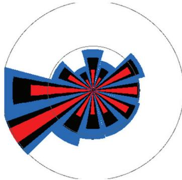
Figure 1: Wind rose diagram shows the wind distribution and likely frequency plotted as 12 sectors according to the European wind atlas1.
