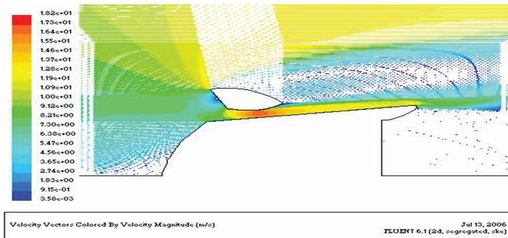
Figure 24: Velocity vectors for wing front angle of attack  $60^\circ$ , in a large grid case.
