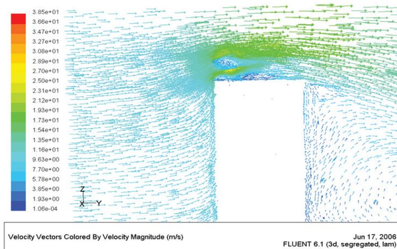
Figure 8: Velocity vectors after installing a wing shape on the same building in figure 7.
