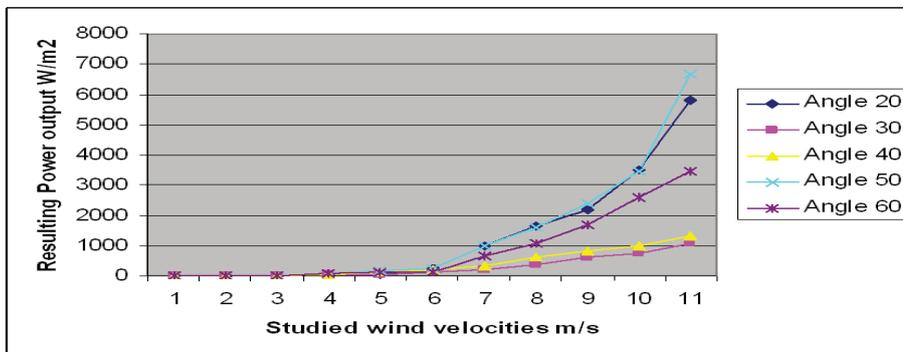
Figure 25: Resulting power output at different wind velocities and angles of wing.
