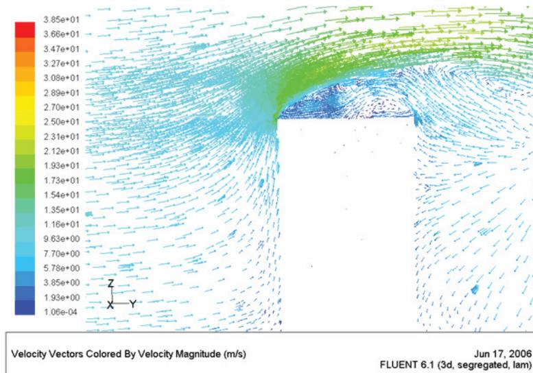
Figure 7: Velocity vectors depicting flow separation on top of a rectangular building.
