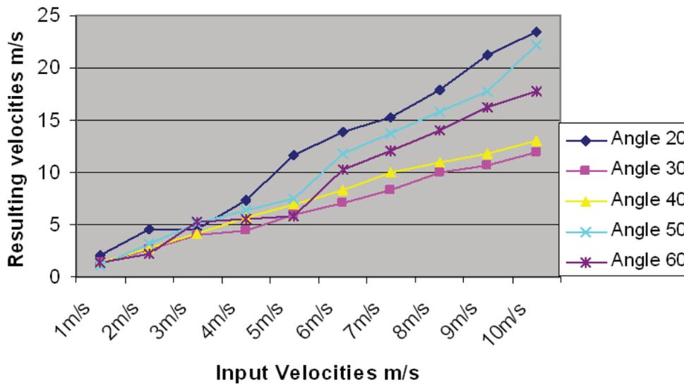
Figure 18: Variation of resulting wind velocities with wing angles at different input wind speed, In Large grid cases.
