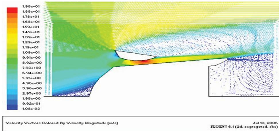
Figure 23: Velocity vectors for wing front angle of attack  $50^\circ$ , in a large grid case.
