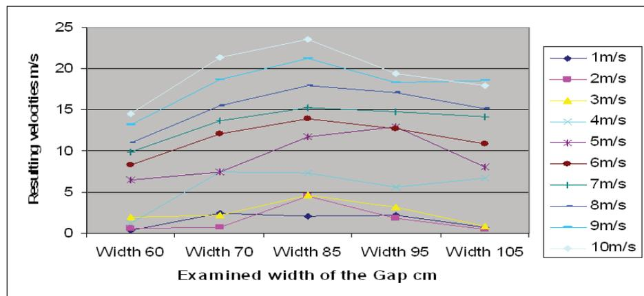
Figure 16: Comparison of the resulting velocities due to examined widths at various tested velocities.
