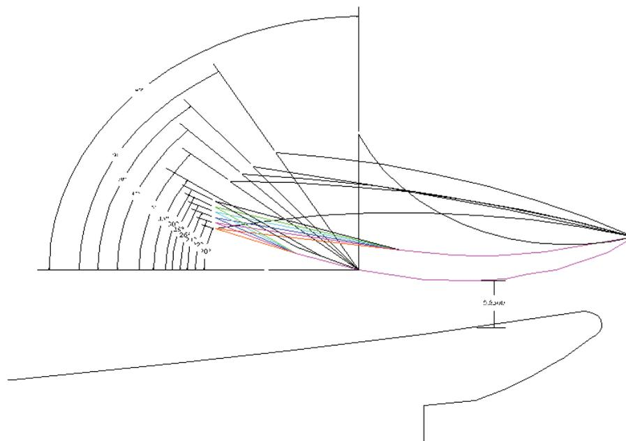
Figure 17: A schematic showing the different opening angles of wind energy capturing wings.
