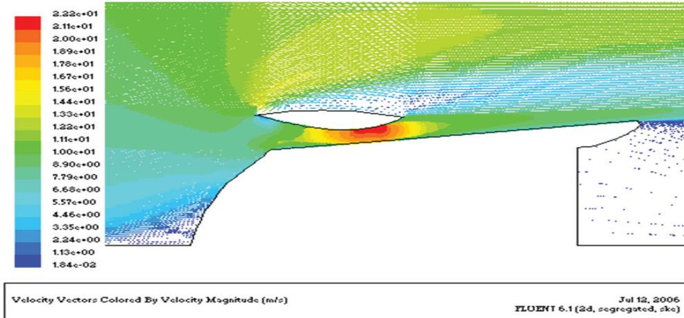
Figure 20: Velocity vectors for wing front angle of attack 20°, in a large grid case.
