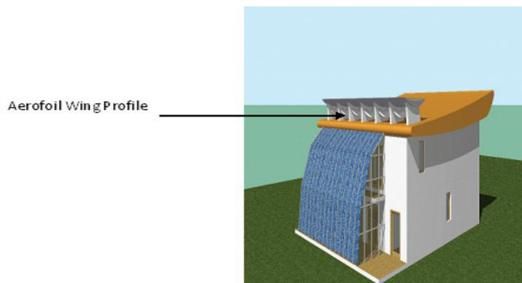
Figure 10: Typical wind turbine integrated in a prototype-detached house, Wing profile on low end of the roof.
